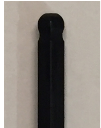
Figure 2: Typical rounded edge flathead screwdriver or ball head hex
