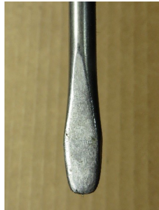
Figure 2: Typical rounded edge flathead screwdriver or ball head hex
