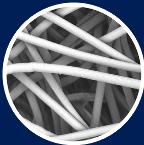
Standard polyester felt magnified 300 times.
