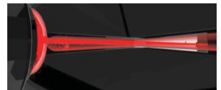
Fig 3. A cast image or shadow created by the contaminant in the oil creates a measurable change in the light intensity.
