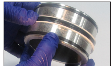
Completed piston seal assembly for a standard V-O-ring
