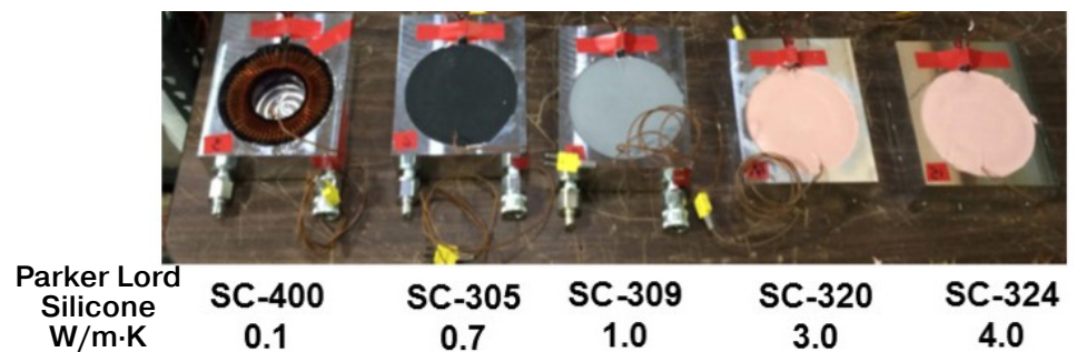
Figure 2: Inductors potted in aluminum cooling plates with each of the Parker Lord potting materials.
