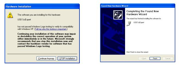
Choose "Continue Anyway", and the driver will finish loading, allowing you to communicate with the LabTec via the assigned Com Port.
