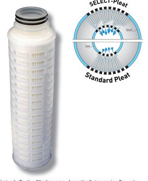
SELECT pleating provides an optimized effective filtration area, dramatically increasing flow rates compared to products with standard pleat format.
