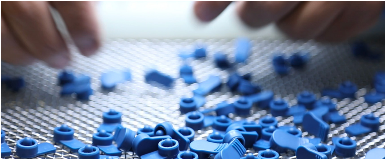
Fig.9. Compression molded silicone profiles
