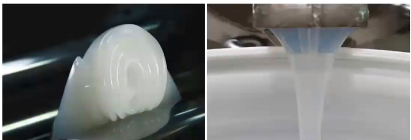
Fig. 3. High consistency rubber (HCR) silicone (left) and liquid silicone rubber (LSR) (right)
