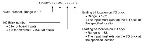
The 6K inputs are read every 2 milliseconds, modified by INLVL and INEN, and debounced with the time specified in INDEB. The inputs specified by INVARI are monitored after they are modified by INLVL and INEN, but before the debounce. Thus, the VARI variable specified by the INVARI command will be updated every 2 milliseconds.
