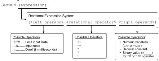
The expression in the PGOWHN command may be specified as a time (dwell) in milliseconds (e.g., PGOWHN(T=2000)), or as inputs or limits matching the specified binary pattern (e.g., PGOWHN(LIM.3=B1) or PGOWHN(2IN.6=B0)). All participating axes will be at rest during a dwell, even if the previous segment had not ended in zero path velocity. In the latter case (limit or input condition), there will be an abrupt change to zero path velocity, until the PGOWHN condition is satisfied.
