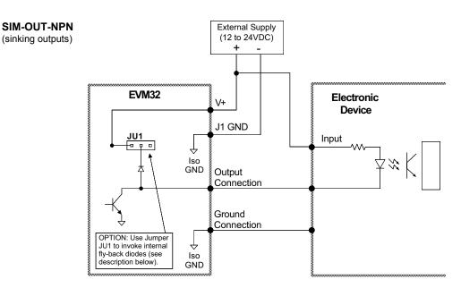
**Fly-Back Diodes**: The SIM card is sent from the factory with jumper JU1 in the "no connect" position (fly-back diodes not used). If you move the jumper to the left-hand position, eight fly-back diodes are invoked, one for each of the 8 output channels. **CAUTION**: If the power supply voltage for the remote device (to which the outputs are connected) is greater than the power supply voltage for the EVM32, <u>do not</u> use the fly-back diodes.
