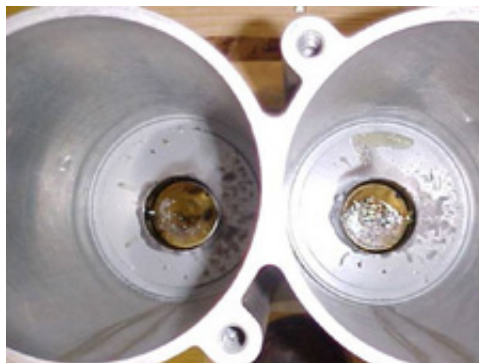
The above pictures show examples of contamination that has been successfully removed by a Parker PCO2 system.
