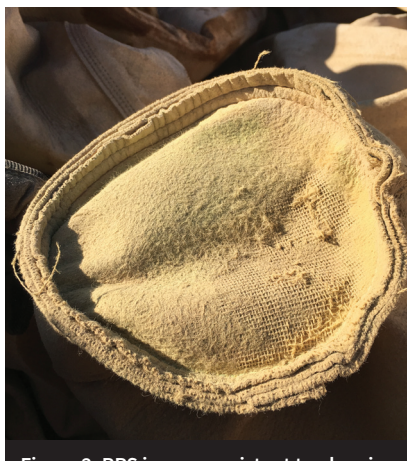
Figure 2: PPS is more resistant to abrasion than fibreglass but not as resistant as aramid media
