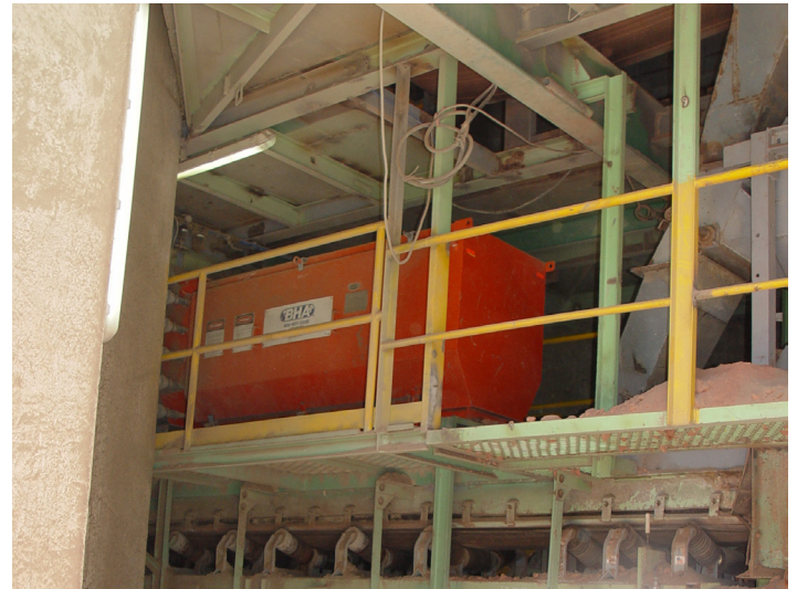
Figure 3: CFS dust collector over conveyor belt underneath clinker silo with overhead restrictions
