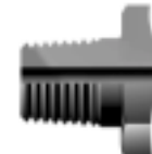
M -ANSI/ASME B1.20.1 External pipe threads
