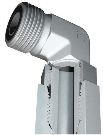
High pressure (700 bar) port configuration
