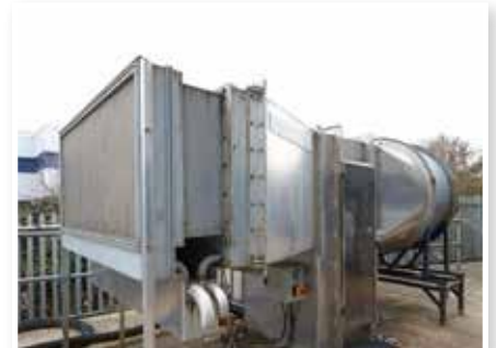
The Neptune test rig allows us to test for water removal capability, a key concern for those located offshore or in a tropical location where heavy rainfall is a factor.
