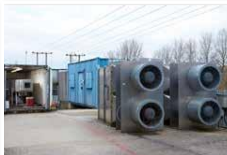
Our outside test rigs allow us to evaluate filters for up to 6 months and measure a variety of factors, including initial DP, fractional efficiency, and reaction to mist and fog.
