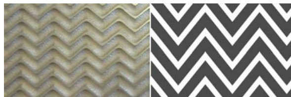
Fig. 7. Heatic PCHE channels (left) – T.I.T. claim for PCHE channels (right).
