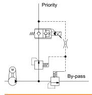
FAP and Logic valves used as a proportional compensated flow control with by-pass. Priority flow is proportionally controlled by the FAP across the compensator. When the priority flow rate is met, the valve allows additional flow available from the pump to by-pass to another function.
