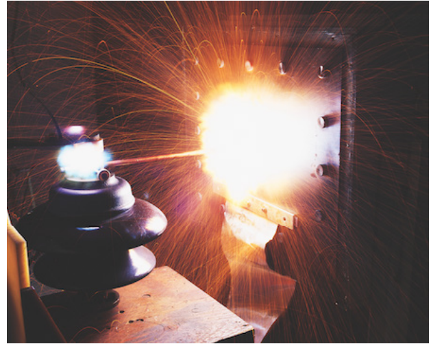
Testing of lightning strike mitigation equipment.
