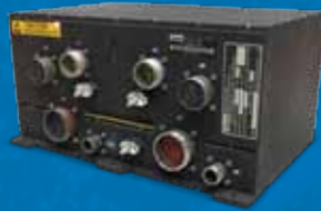
F-35 actuation control electronics
