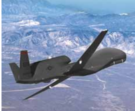
UAV aircraft like Northrop Grumman's RQ-4 Global Hawk rely on SprayCool® thermal management technology for electronics cooling in unpressurized space.
