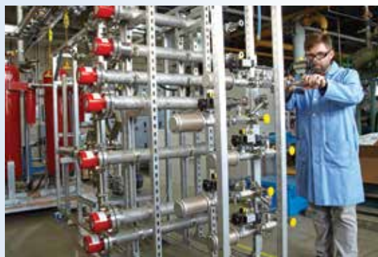
An air separation module endurance test rig at our Fluid Systems Division in Irvine, California.
