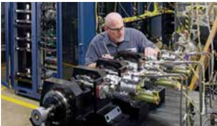
Eight complete airframe flight control SILs perform cockpit-to-control surface functions.
