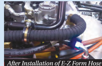
After Installation of E-Z Form Hose
