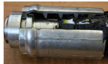
Improper insertion depth
