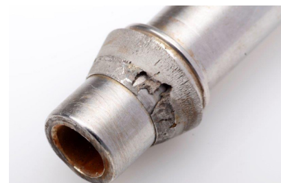
Figure 1. These twin ferrule compression fittings - made from 316 stainless steel - were removed from a 6MO tubing run that had been in service offshore for around nine months - and illustrate the potential problems of making decisions about fittings purely on cost grounds alone.
