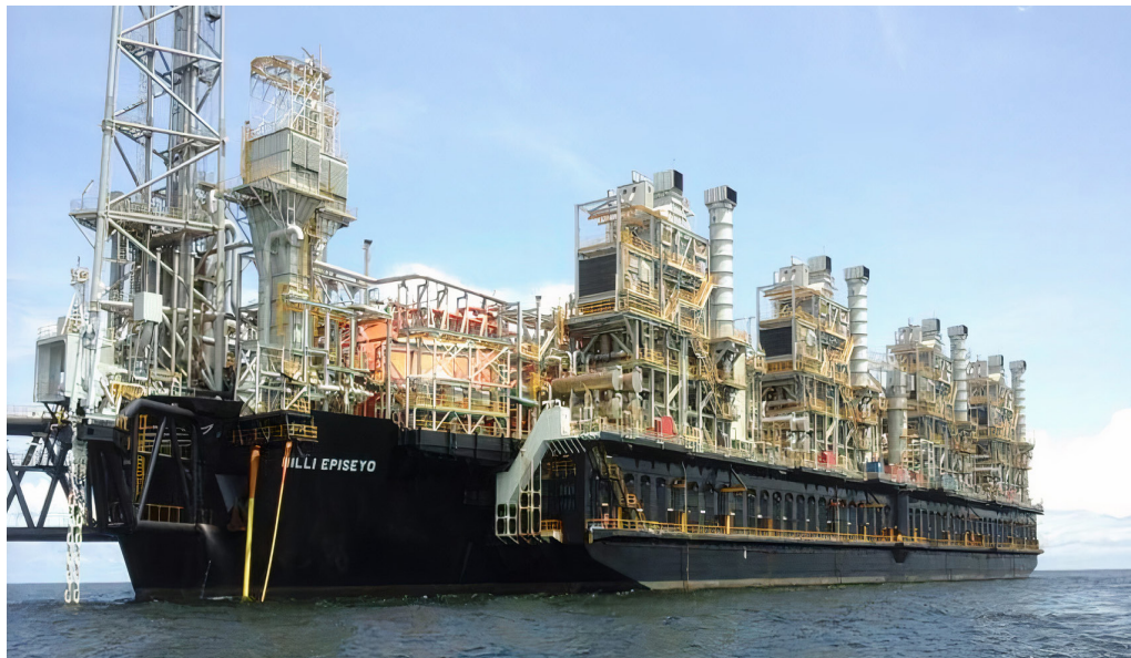
Fig. 1. The 4 x 0.6 million tpy train Golar Hilli Episeyo FLNG production vessel.
