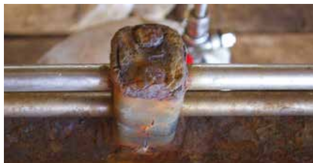
Crevice corrosion between the tube/tube trap interface.
