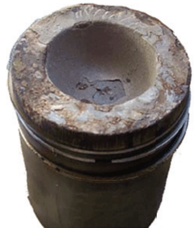
A piston coated in silica deposits
