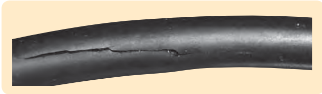
Figure 10-4: O-Ring Damaged by Explosive Decompression
