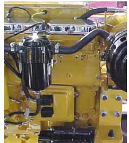
Pictures below: (left) Cummins QSM11 marine engine with CCV cutaway. (right) Caterpillar 3196 marine engine with Racor CCV/AF System.
