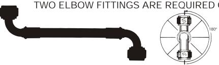
MEASURING: When installations require hose assemblies with elbow fittings on both sides, hold the assembly so that the nearest fitting is pointing in the 6 o'clock position. Measure angle between fitting, counterclockwise. Both fittings pointing to 6 o'clock to be specified as zero degrees (0°)
