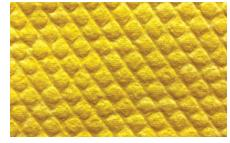
Exclusive synthetic media with graduated dimples to hold two times more dust and reduce initial resistance.
