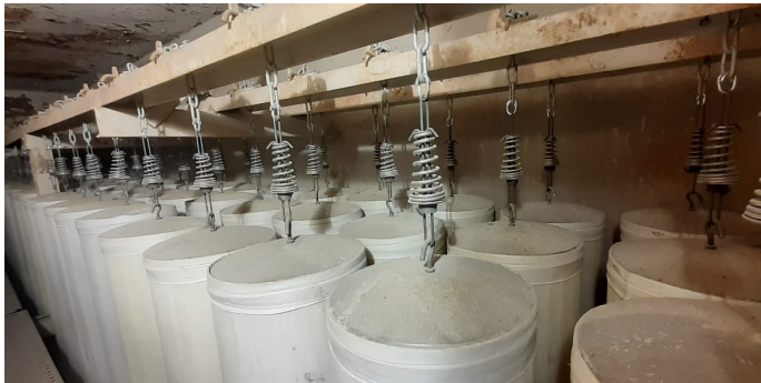
Conical stainless-steel springs at the top end absorb shock and help manage tension during the cleaning cycle.
