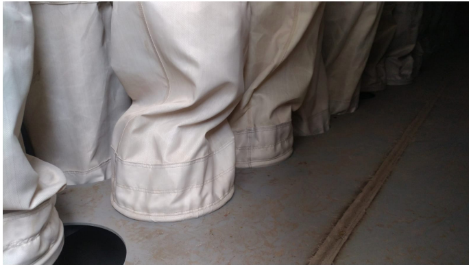
Replacing user-adjusted clamps and thimbles with pre-fitted snapbands cuts bag install time and ensures accurate pressure.
