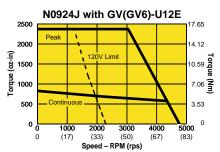
Solid lines represent 240VAC operation, continuous and peak. Dashed lines represent performance using 120VAC input. Speed/torque curves may vary +/- 10%.
