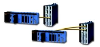
Gemini with the 6K Motion Controller: Up to 8 axes of the Gemini GV or GT Drives can be accurately controlled with Compumotor's revolutionary 6K Motion Controller.
