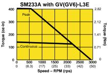
Solid lines represent 120VAC operation, continuous and peak. Speed/torque curves may vary +/- 10%.
