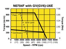
Solid lines represent 240VAC operation, continuous and peak. Dashed lines represent performance using 120VAC input. Speed/torque curves may vary +/- 10%.
